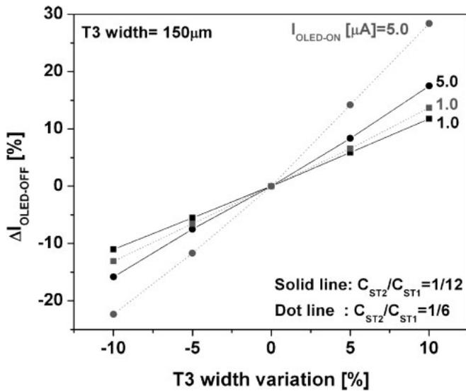
Fig. 7. Variation of  $I_{\text{OLED,OFF}}$  as a function of T3 width deviation.
