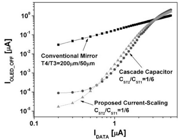
Fig. 5. Comparison of  $I_{OLED\_OFF}$  vs  $I_{DATA}$  among conventional current-mirror, cascade-capacitor, and proposed pixel electrode circuits.
