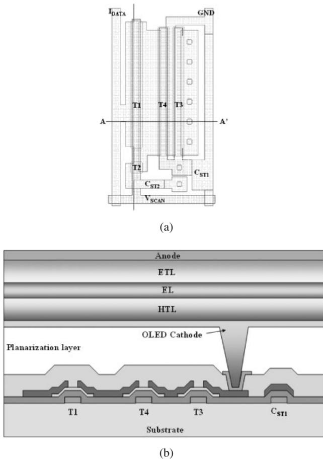
Fig. 9. (a) Schematic top views and (b) cross sections of proposed a-Si:H pixel electrode circuit.
