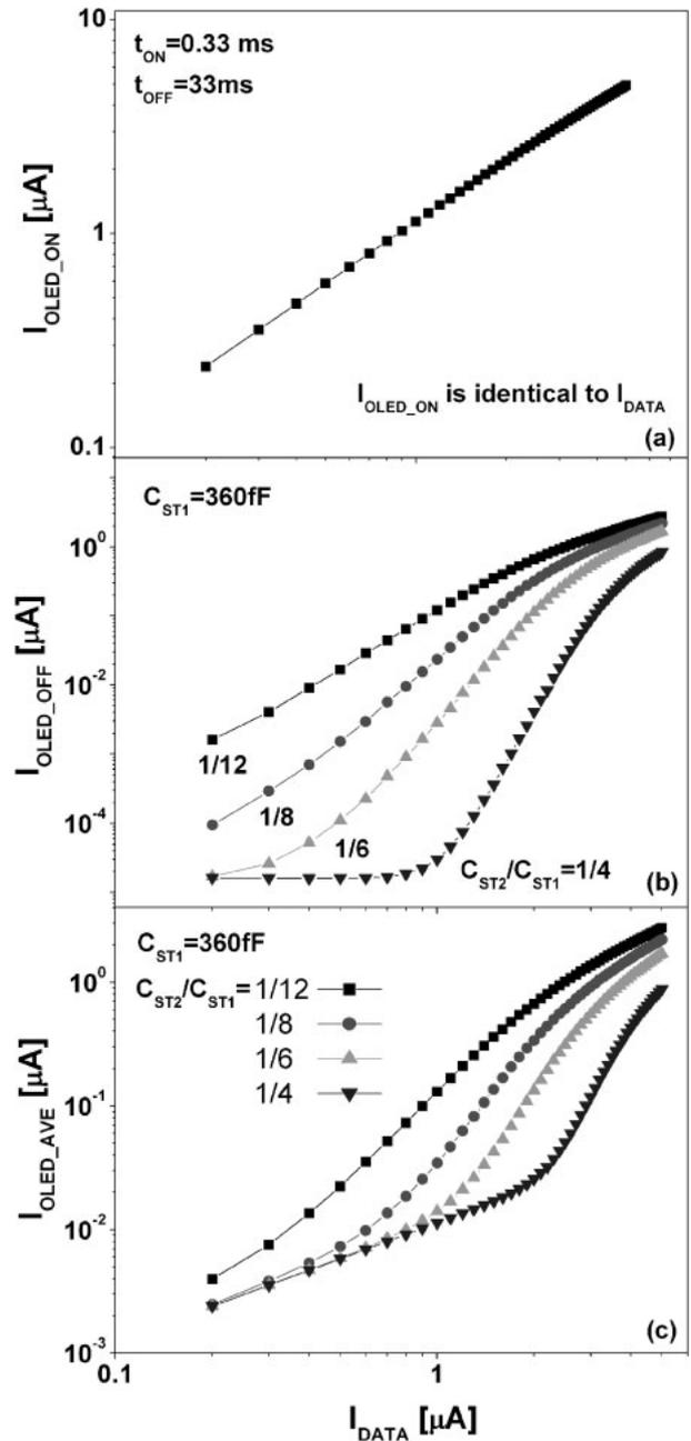
Fig. 3. Variation of the simulated  $I_{OLED\_ON}$ ,  $I_{OLED\_OFF}$ , and  $I_{AVE}$  as a function of  $I_{DATA}$  for various  $C_{ST2}/C_{ST1}$  ratios.
