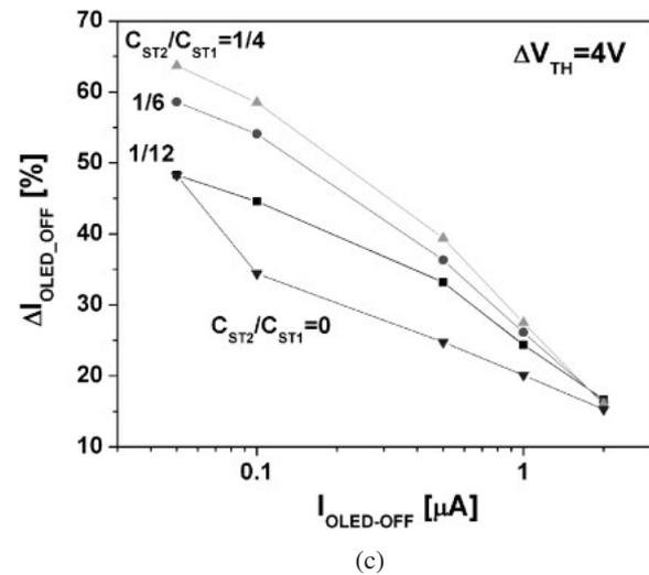
Fig. 6. (a) Changes of transfer curve at  $V_{DS} = 30$  V, and (b) variation of  $\Delta I_{OLED\_OFF}$  as a function of TFT threshold voltage shift. (c)  $\Delta I_{OLED\_OFF}$  VS OLED current during display operation OFF-state for different  $C_{ST2}/C_{ST1}$  ratios when  $\Delta V_{TH} = 4$  V.
