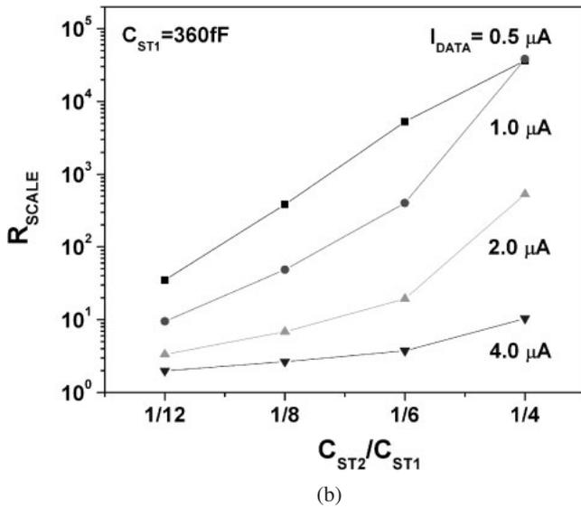
Fig. 4. Variation of the current scaling ratio as a function of (a)  $I_{DATA}$  and (b) ratio of storage capacitances for the proposed pixel circuit.
