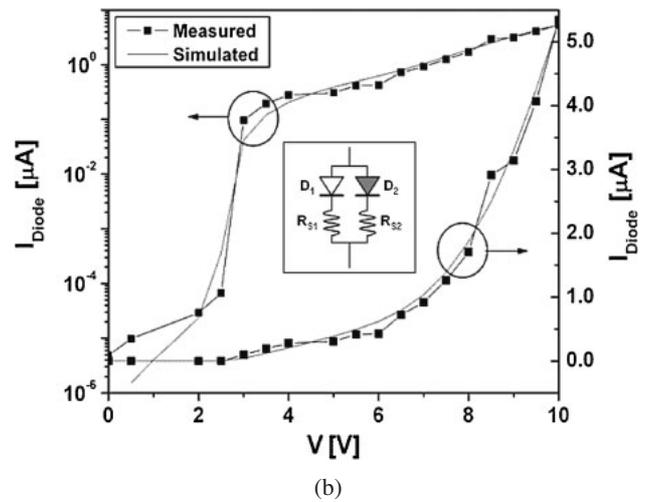
Fig. 2. Measured and simulated (a) transfer characteristics of a-Si:H TFT (b) current–voltage characteristics of white PLED. The equivalent circuit model of white PLED for simulation is shown in insert.
