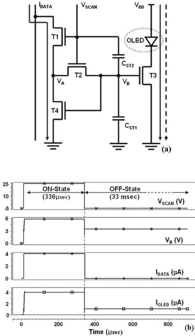
Fig. 1. Schematic of (a) the cascaded-capacitor current mirror pixel electrode circuit and (b) operational waveforms simulated by HSPICE.
